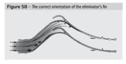
Note: Please ensure the correct orientation of the eliminator's fins.
