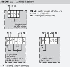
U1, U2 - single-phase motor supply terminals 1f - 230V/50Hz
