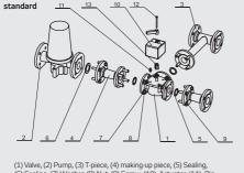
(1) Valve, (2) Pump, (3) T-piece, (4) making-up piece, (5) Sealing, (6) Sealing, (7) Washer, (8) Nut, (9) Screw, (10) Actuator, (11) Pin, (12) Fixing screw, (13) Adapter
