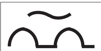
If the property has an earth-leak circuit breaker, the unit must be fitted with a separate earth-leak circuit breaker of type B which also works if there are DC components. See the symbol.
