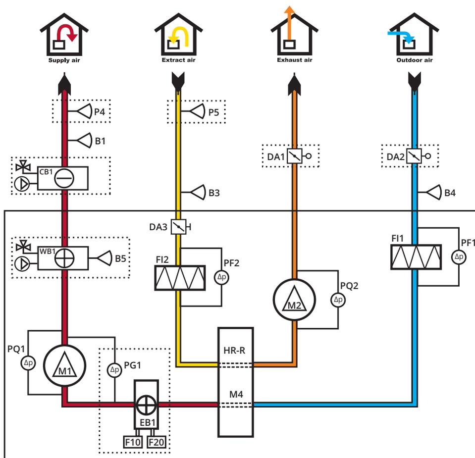
The unit can only have one heating battery - water or electric.
