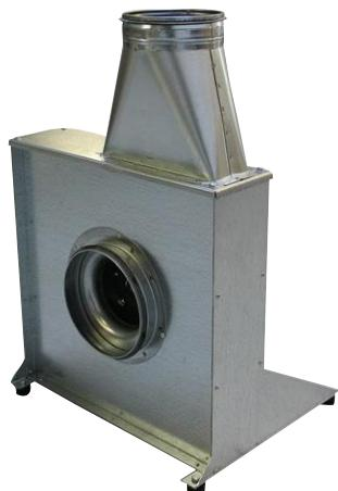
Centrifugal fan with closed wheel with backward curved blades and direct driven flange motor. The MHF-fan is used for industrial process extraction. The MHF-fan delivers a high pressure and is ideal for PID/constant pressure regulation.
