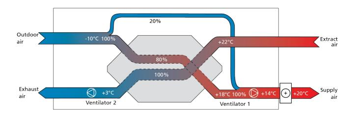
The heat exchanger has two forms of frost protection: temperature-controlled or pressure-controlled. The actual de-icing can take place in several ways, depending on whether an after heating coil has been fitted.
