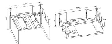
The VEX330 Ceiling unit with hinged or sliding door is available as a LEFT or RIGHT model. The drawing below shows the solution with a hinged door system.
