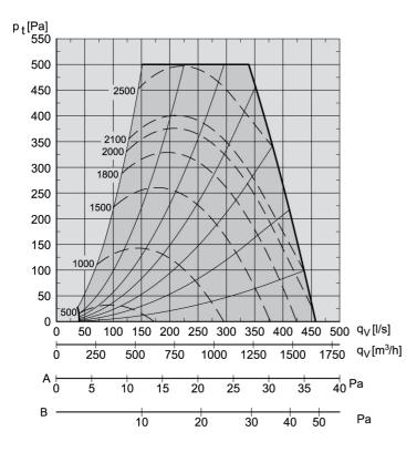
Capacity curve with Coarse 85% filters (M5)
