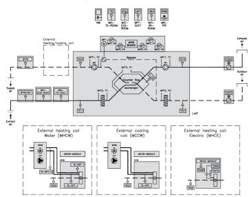
With EXact2, HCW can either be connected directly to the main PCB or via the MHCW module as shown here. If the distance between the unit and the HCW is less than 10m, the connection can be made directly on the main PCB.
