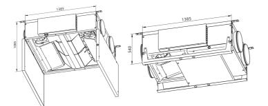
The VEX330 Ceiling unit with hinged or sliding door is available as a LEFT or RIGHT model. The drawing below shows the solution with a hinged door system.
