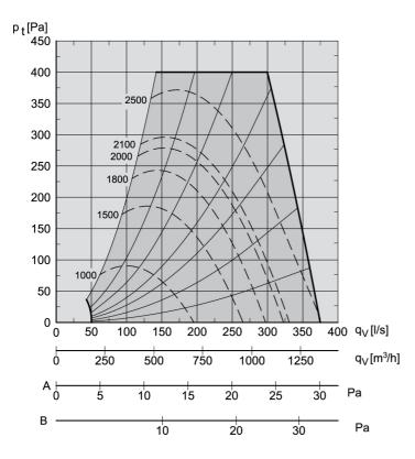
Capacity curve with Coarse 85% filters (M5)
