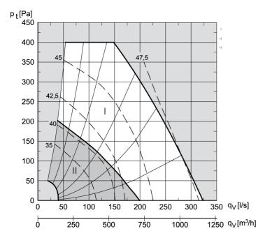
Sound output level Suction side (outdoor air/extract air):  $L_{W1} = L_{WA1} + K_W$  $L_{WA1}$  read Sound output level Surroundings:  $L_{W3} = L_{WA3} + K_W$  $L_{WA3}$  read Sound output level Pressure side (supply air/exhaust air):  $L_{W2} = L_{WA2} + K_W$   $L_{WA2}$  read Sound output level at 1 m distance Surroundings:
