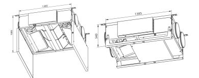
The VEX320 Ceiling with hinged or sliding door is available as a LEFT or RIGHT model. The drawings below show the solution with a hinged door system.
