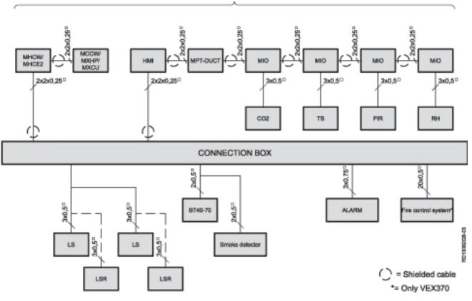
Max. 200 m cable connection in total The sequence of the modules is unimportant
